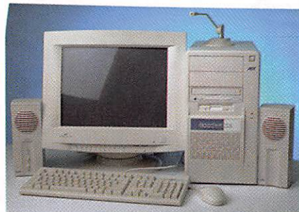
The Advantage 9314 is built like a vault, with a heavy steel chassis and case.
