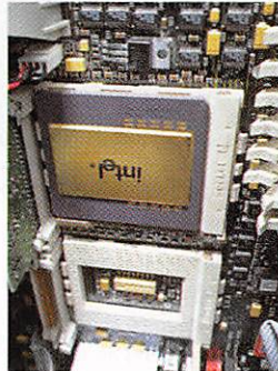
The HP Vectra XW features sockets for two 200MHz Pentium Pros. We've removed the heat sink for this shot.
