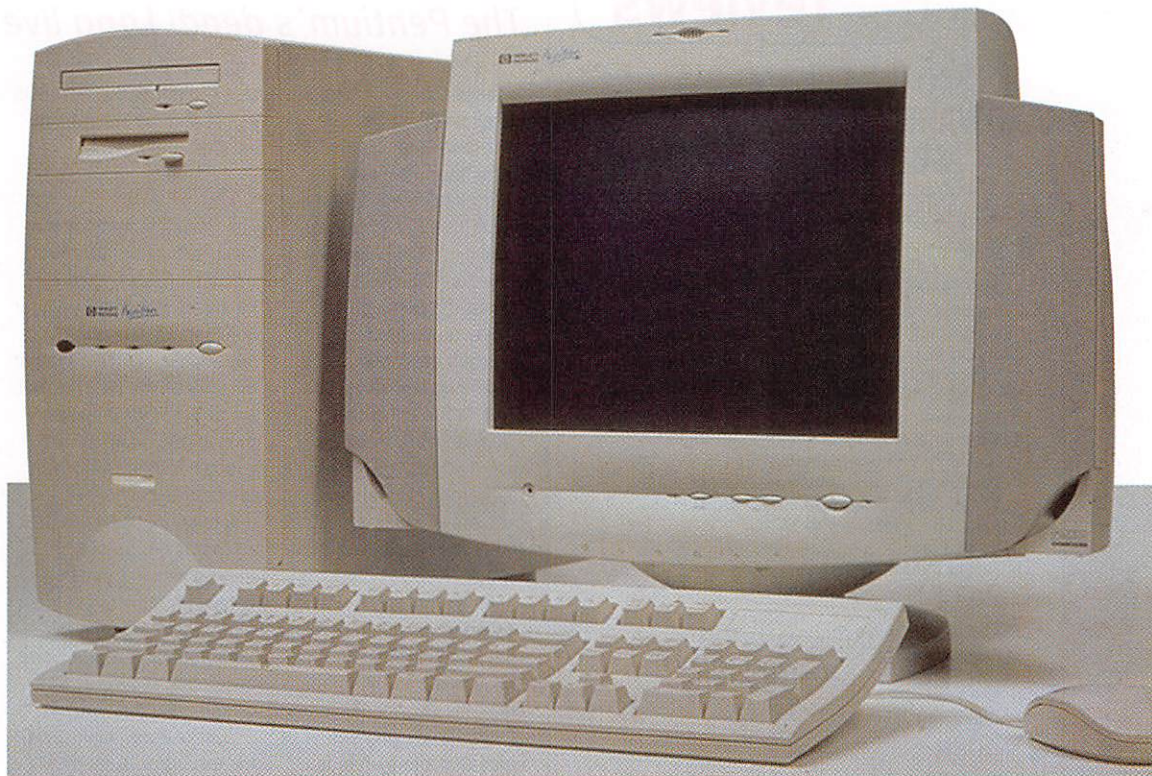
Hewlett-Packard's Pavilion 7295V keeps the same exterior and expansion options as last year's models, but pumps up the power with components, including a 200MHz Pentium, 256K of pipeline burst cache, and wavetable audio.
