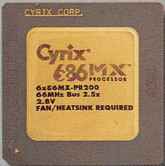
Cyril 6x86MX-PR200 Clock Speed 166MHz (2.5x multiplier) System Bus Speed 66MHz PCI Bus Speed 33MHz
